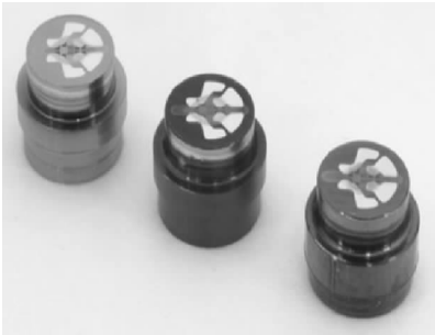
图 5 带沉积应变计的玻璃隔膜的外观 [45] Fig.5 Appearance of glassy diaphragms with deposited strain gauge [45]
